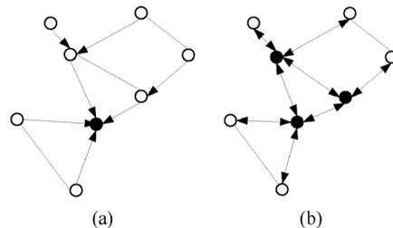
Fig. 1. Sensor Pairing. (a) centralized. (b) decentralized.
