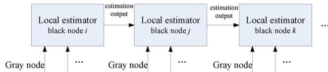
Fig. 3. Decentralized source localization architecture.
