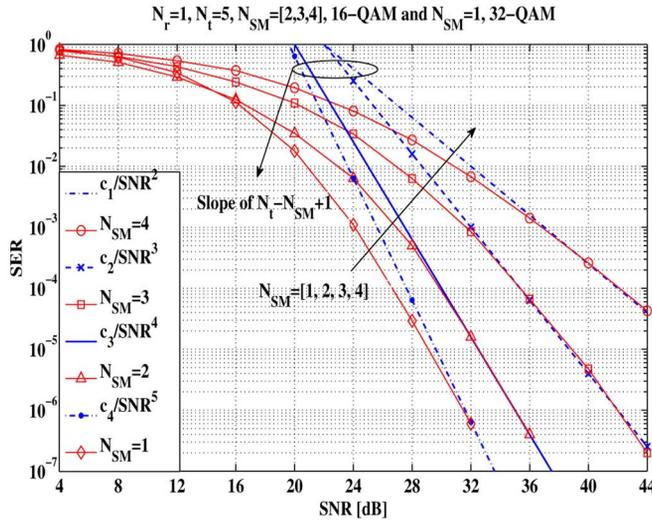
Fig. 2. SER performance of the SM system having  $N_r = 1$ ,  $N_t = 5$  and employing 16-QAM signal set for  $N_{SM} \in [2, 3, 4]$ .
