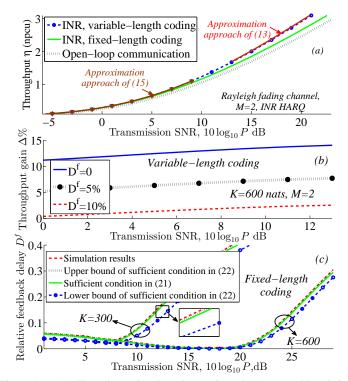
Figure 1. (a): Throughput, (b): throughput gain and (c): acceptable relative feedback delay vs SNR, M = 2. In subplot (a), both the number of information nats and the sub-codewords' length are optimized in terms of throughput. In subplots (b) and (c), K = 600 and K = 300, 600 nats, respectively.
