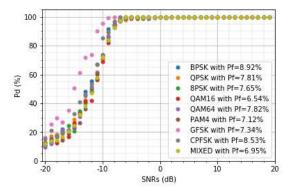
Fig. 3. Impact of modulation scheme on performance.
