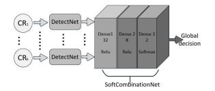
Fig. 5. DL based cooperative detection system design.
