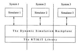
Figure 1. Dynamic Simulation Backplane architecture
