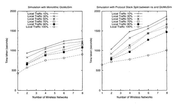
Figure 4. Simulation running time with 200 wireless nodes in each wireless network
