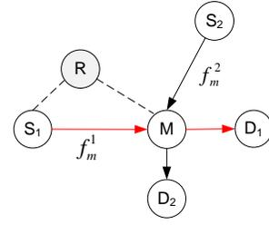
Fig. 2. The relay node in cooperation with a single unidirectional flow.
