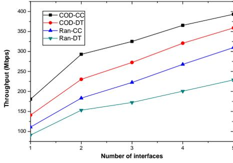
Fig. 13. Simulation results with total throughput.
