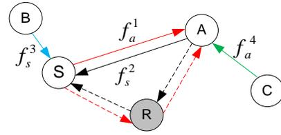
Fig. 5. Relay node in cooperation with bidirectional flows.
