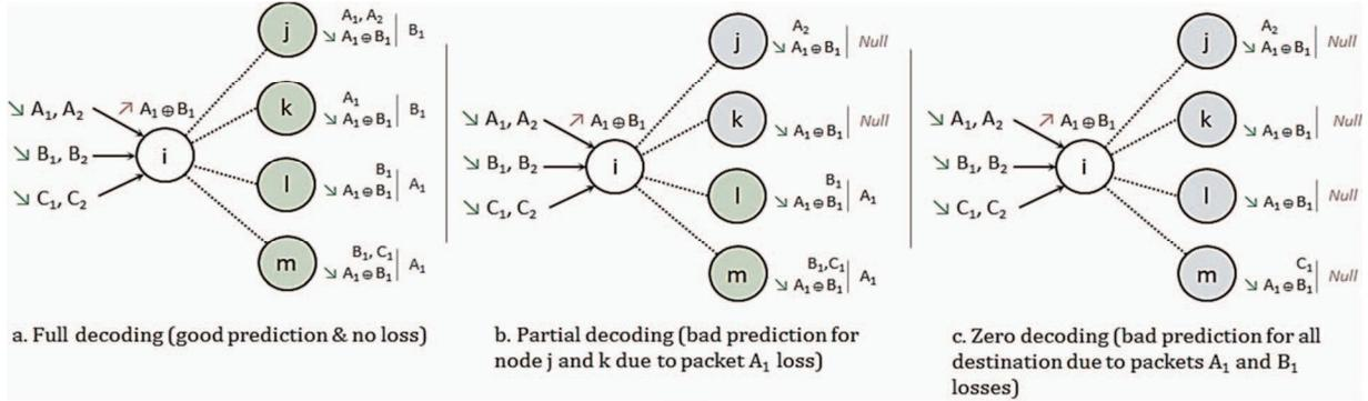
Figure 2 - Packet loss impact on coding efficiency illustration
