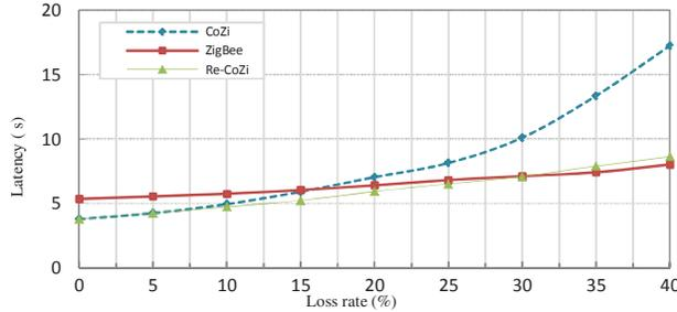
Figure 4 – Latency versus packet loss rate
