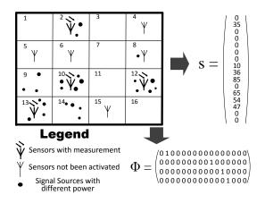
Fig. 1. A demo of the system with the corresponding signal vector  $\boldsymbol{s}$  and measurement matrix  $\boldsymbol{\Phi}.$
