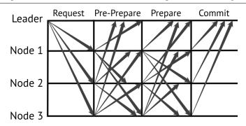
Fig. 2. An illustration of how BA protocol works with replicated nodes.
