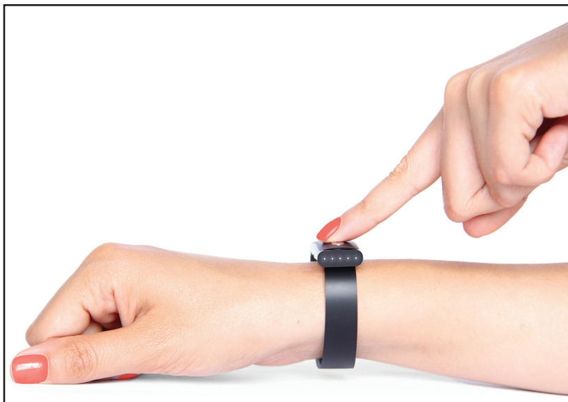
Users touch the Nymi wristband to activate it. The band then generates electrocardiogram readings, which it uses to authenticate wearers to computers, applications, and other systems.
