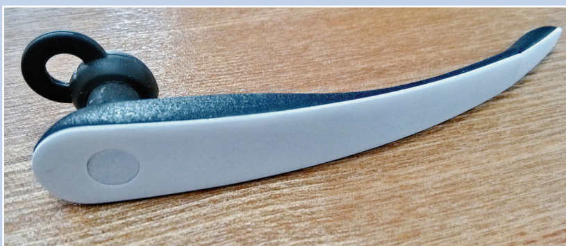
The Vigo headset tracks wearers’ eyeblinks and head motions to determine if they are becoming less alert. If so, the device tries to get users to focus via a flashing light, earpiece vibrations, or an alarm.
