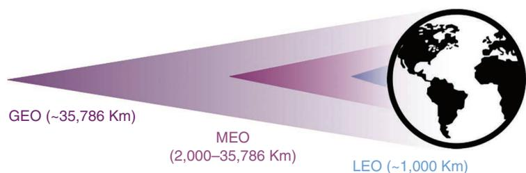
FIGURE 3. The GEO, MEO, and LEO orbitals.
