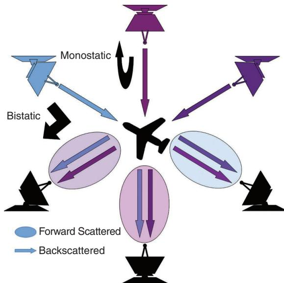
FIGURE 2. The monostatic, bistatic, and multistatic radar configurations.
