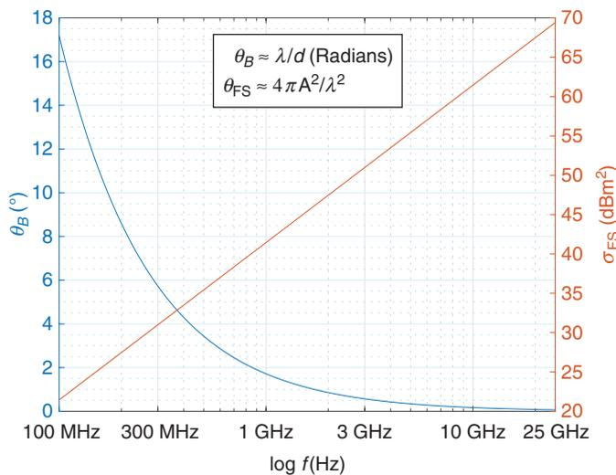
**FIGURE 4.** The forward scattering system trade space: the forward scatter RCS ( $\sigma_{FS}$ ) and angular width of scatter ( $\theta_B$ ) for an idealized medium-sized airborne target with  $A = 10 \text{ m}^2$  and  $d = 10 \text{ m}$ , where  $A$  is the cross-sectional area of the target and  $d$  is the greatest linear distance to the target.
