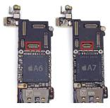
Yes, well this is clearly the biggest difference. The iPhone 5c has the A6 CPU manufactured using a 32-nm process on a 96.71-mm<sup>2</sup> die, ARM-7 dual core running at 1.3 GHz. There is also a 266-MHz graphics processing unit (GPU) **<AU: Please check whether GPU is spelled out correctly.>** and
