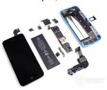
Just like in the iPhone 5, the display assembly is the first component out of the phone, simplifying screen replacements.
