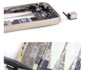
We next uncover the iSight camera. According to our friends at Chipworks, "the DNL markings are consistent with the markings on the camera modules housing the Sony IMX145 we saw in the iPhone 4s and the iPhone 5. The marks on the side of the module are different, but our industry insiders tell us this is Sony's again."
