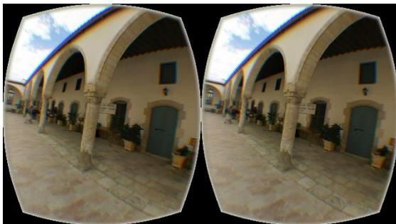
Figure 5 - Ray-casted ground truth. All stimuli was synthesised and rendered as if it would be displayed to a real user in an HMD, down to the per-colour distortions to compensate for chromatic aberration in the lenses. This image would have been compared to a real frame such as that shown in Figure 2.
