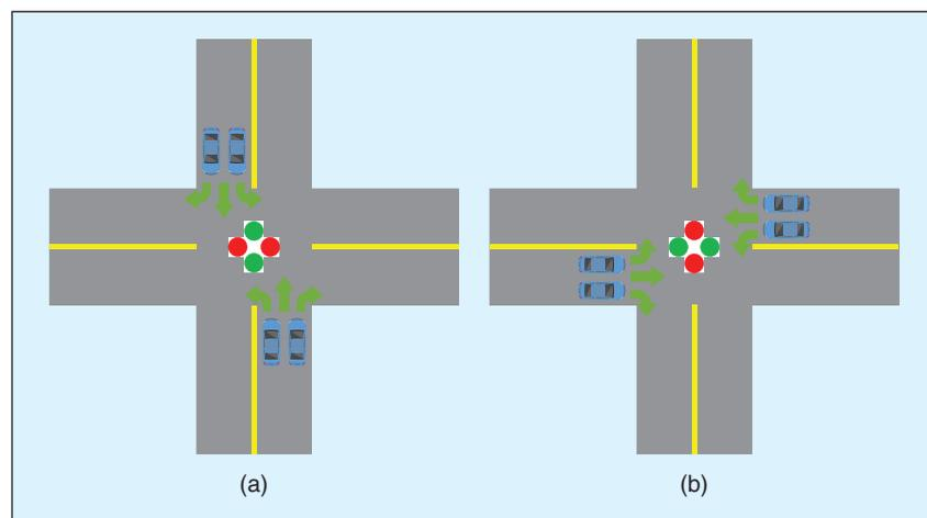
**FIGURE 3** Two examples of a traffic light signal phase. (a) Signal phase for the up-down direction. (b) Signal phase for the left-right direction.
