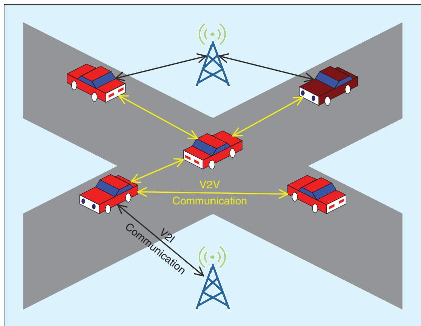
**FIGURE 2** Example of a vehicular network with V2I and V2V communications.
