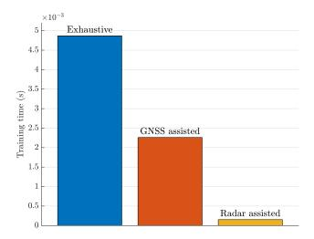
Fig. 3: The overhead of beam-search in phased-array based analog mmWave system with 64 antennas at the RSU and 16 antennas at the vehicle. The symbol duration is  $4.75 \,\mu\text{s}$ . The exhaustive beam-search requires that 1024 beam-pairs be tested with training time  $4.87 \,\text{ms}$ . This is reduced to 475 beam-pairs (2.3 ms) using GNSS based position information, and to 32 beam-pairs (0.15 ms) using RSU mounted radar-based positioning.
