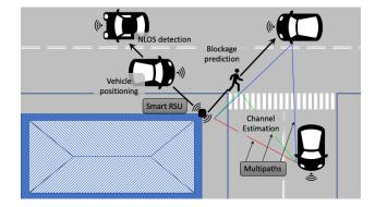
Fig. 2: Sensors at infrastructure can help the mmWave communication by vehicle positioning, blockage mitigation, NLOS detection, and channel estimation.
