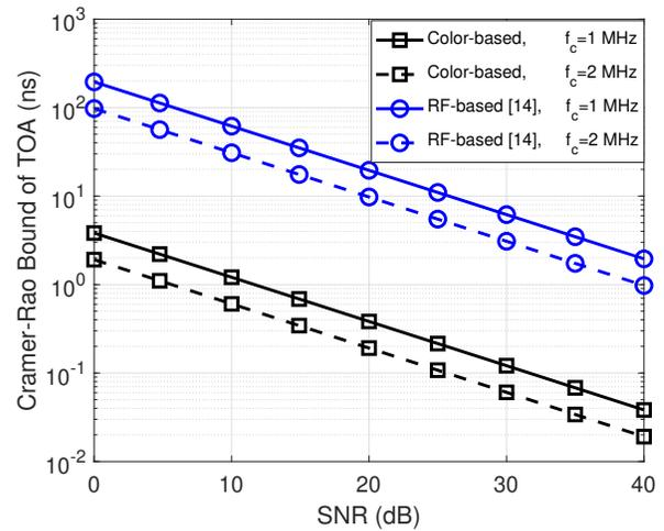
Figure 5: The comparison of ToA performance for proposed color-based and conventional RF-based technique [14].
