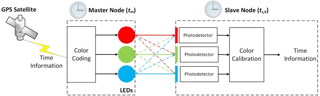
Figure 2: The architecture consists of a master clock, slave clocks, and a GPS satellite serving as the time source for color-based time synchronization distribution.
