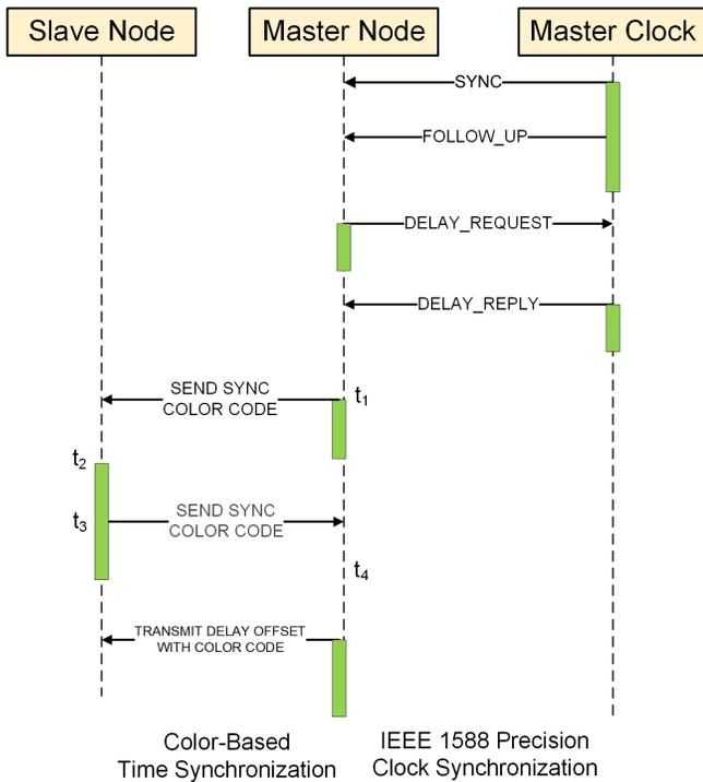
Figure 4: The signalling diagram of the proposed solution.
