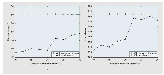
**Figure 6.** Scatternet formation delay vs. scatternet formation timeout: a) maximum scatternet formation delay; b) total scatternet formation delay.
