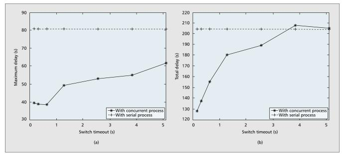
**Figure 5.** Scatternet formation delay vs. switch timeout: a) maximum scatternet formation delay; b) total scatternet formation delay.
