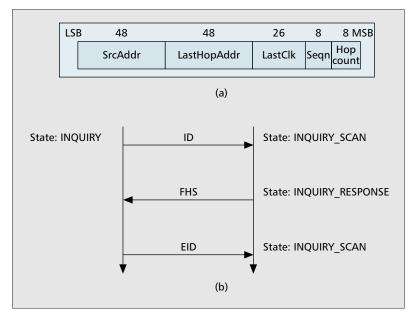
**Figure 2.** Modified Inquiry with EID packet: a) EID packet format; b) modified Inquiry process.
