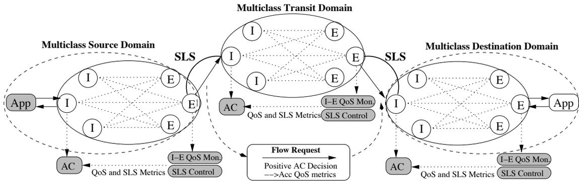
Fig. 4. Distributed monitoring-based AC approach
