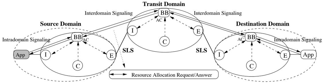
Fig. 2. Centralized AC using BBs
