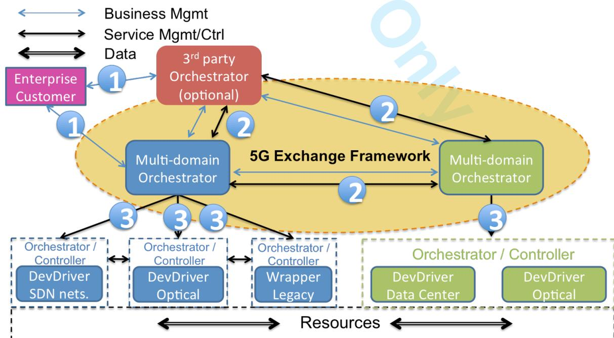
Figure 2 Simplified conceptual architecture of the 5G Exchange
