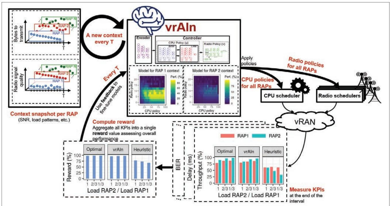
FIGURE 3. AI-aided approach to joint computing/radio resource orchestration [4].
