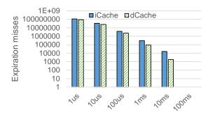
Fig. 5: Average expiration misses for different retention times.
