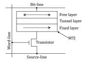
Fig. 1: STT-RAM basic cell structure
