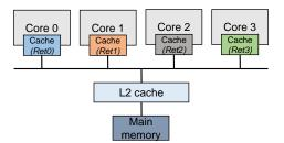
Fig. 12: Illustration of proposed asymmetric retention caches. The L1 caches feature different retention times to satisfy a variety of execution requirements.
