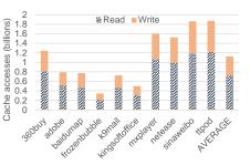
Fig. 2: Read-write ratio for data cache memory accesses
