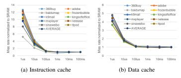
Fig. 6: Instruction and data cache miss rates for different retention times normalized to SRAM
