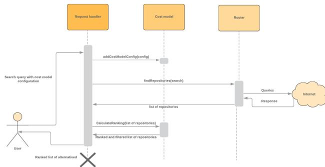
Fig. 5. Control flow for user query [26]
