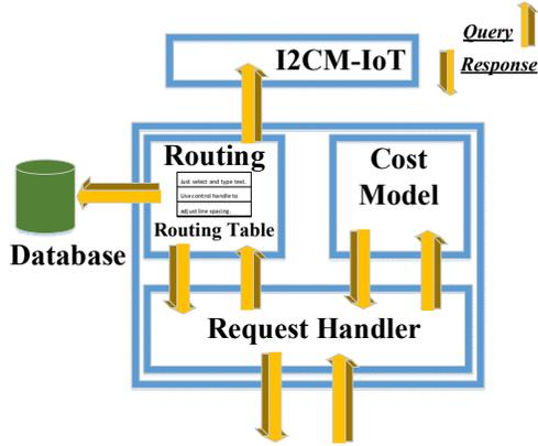
Fig. 4. Internal architecture of an I2CM-IoT [26]
