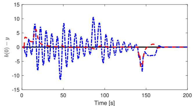
Fig. 5: Case 1: Tracking error for the old (blue) and new (red) methods.
