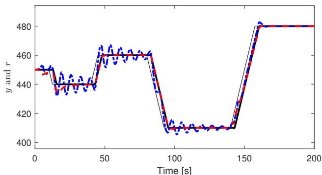
Fig. 4: Case 2: Reference signal  $y_r$  (thick black) and measured downhole pressure for the new (red) and old (blue) methods. Also plotted is the input  $r$  to the reference model (thin black).
