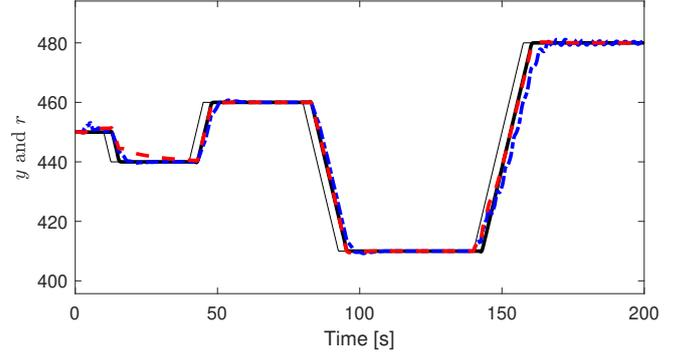
Fig. 1: Case 1: Reference signal  $y_r$  (thick black) and measured downhole pressure for the new (red) and old (blue) methods. Also plotted is the input  $r$  to the reference model (thin black).
