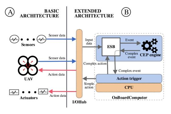
Figure 1. An autonomous-UAV (unmanned aerial vehicle) architecture for remote sensing and intelligent decision making. The hardware components are orange; the software components are blue. ESB = enterprise service bus; CEP = complex event processing.
