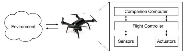
Fig. 3: Closed-loop data flow in a MAV. Information flows from sensors collecting environment data into the MAV’s compute system, down into the actuators and back to the environment.
