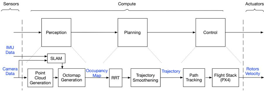
Fig. 5: High-level application pipeline for a typical MAV application. The upper row presents a universal pipeline that all our MAVBench applications follow, which involves *perception*, *planning* and *control*. The lower row presents how a specific workload in MAVBench (e.g. package delivery) maps to the universal high-level application pipeline.
