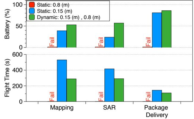
Fig. 19: Switching between OctoMap resolutions dynamically leads to successfully finishing the mission compared to 0.80 m. It also leads to battery life improvement compared to 0.15 m. The  $y$ -axis in the top graph is the battery left on the drone upon mission completion.
