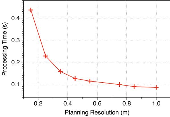
Fig. 18: Reduction in OctoMap resolution (accuracy) can be traded off with processing time. Increasing the  $x$ -axis means larger voxels to represent the space more coarsely (less accurately). A 6.5X reduction in resolution results in a 4.5X improvement in processing time.
