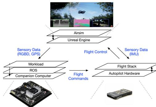
Fig. 4: Architectural overview of our closed-loop simulation.
