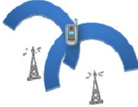
Figure 2. Illustration of overlapping timing advance range rings (From [8]).
