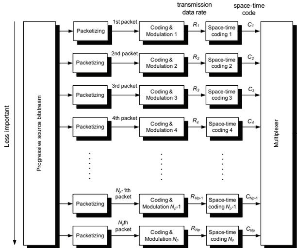
Fig. 2. Progressive source transmission system combined with open-loop MIMO techniques.  $R_i$  and  $C_i$  denote the transmission data rate and the space-time code assigned to  $i$ th packet, respectively ( $1 \leq i \leq N_P$ ).
