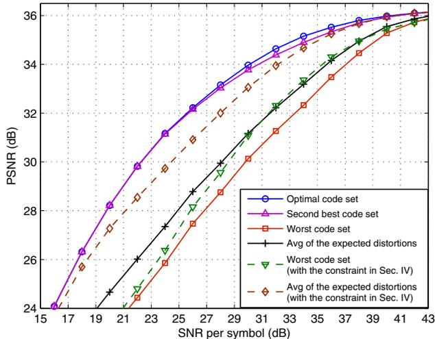
Fig. 5. The PSNR performance of the optimal set of space-time codes and suboptimal ones for the transmission of progressive 8 bpp  $512 \times 512$  Lena image for  $2 \times 2$  MIMO systems in i.i.d Rayleigh fading channels.
