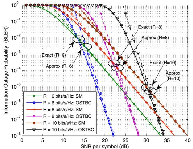
Fig. 3. The exact and high SNR approximate outage probabilities of OSTBC and SM with a ZF receiver for  $2 \times 4$  MIMO systems in i.i.d. Rayleigh fading channels. Solid curves denote the exact outage probabilities, and dashed curves denote the high SNR approximate outage probabilities. The exact and approximate crossover points are marked with circles.
