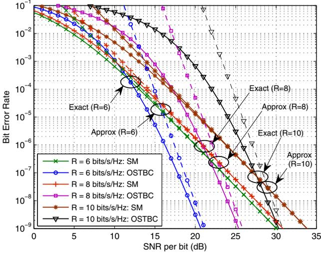
Fig. 4. The exact and high SNR approximate uncoded BERs of OSTBC and SM with a ZF receiver for  $2 \times 4$  MIMO systems in i.i.d Rayleigh fading channels. Solid curves denote the exact BERs, and dashed curves do the high SNR approximate BERs. The exact and approximate crossover points are marked with circles.
