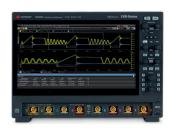
Fault Hunter feature automatically analyzes the normal signal for 30 seconds and initiates advanced triggers to find rare or random signal faults. The EXR-Series' automatic, one-button launch to find physical layer signal anomalies speeds design and troubleshooting efforts, adding efficiency and expertise. Infiniium users can analyze data anywhere with the advanced Infinium Offline software.
