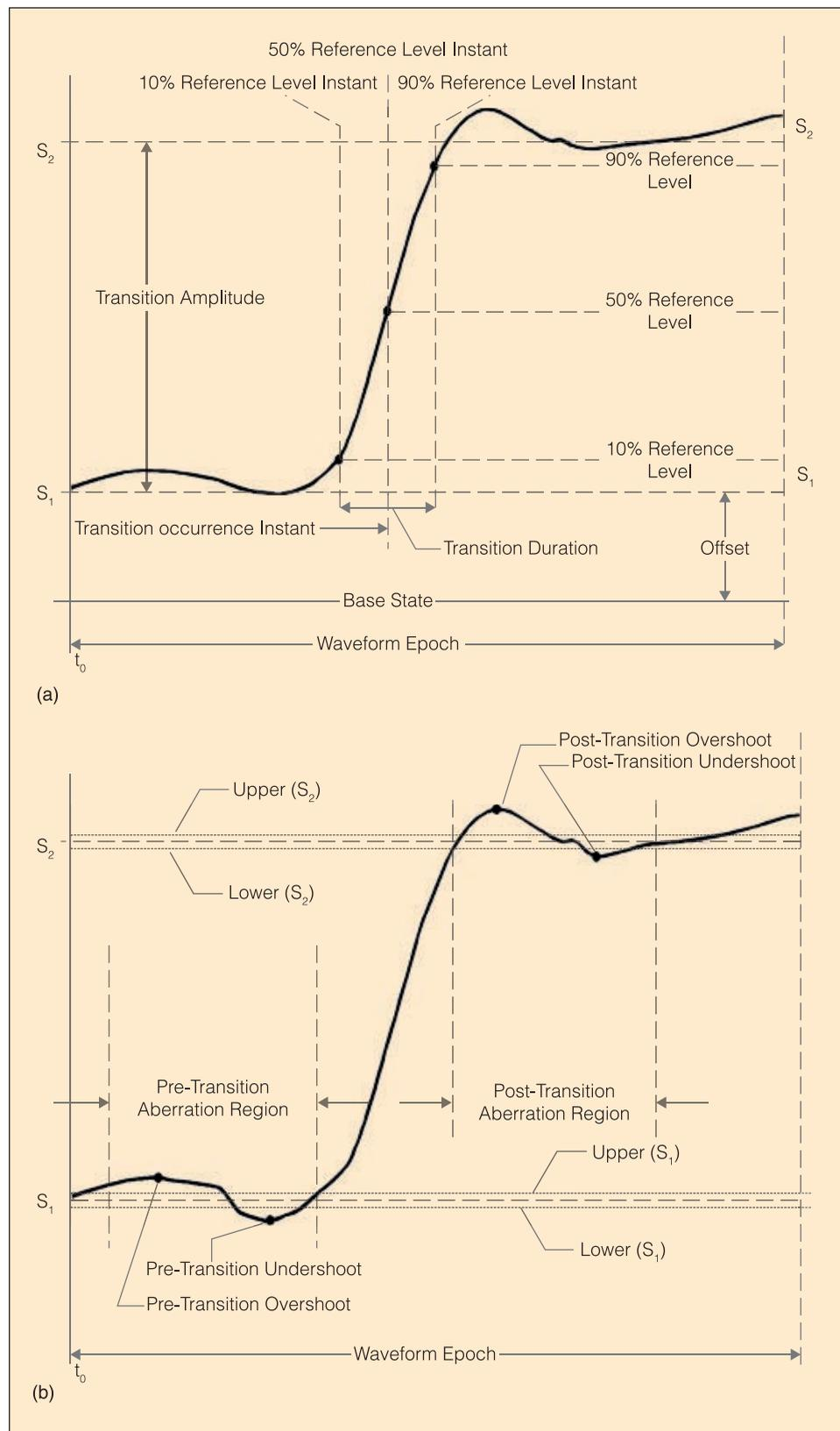
**Fig. 2.** Two plots displaying various parameters used to describe the characteristics of a waveform. The plot on the left shows the fundamental waveform parameters on which all other parameters are derived. The plot on the right shows the parameters that are used to describe aberrations of a waveform (from [7], ©2020 IEEE).
