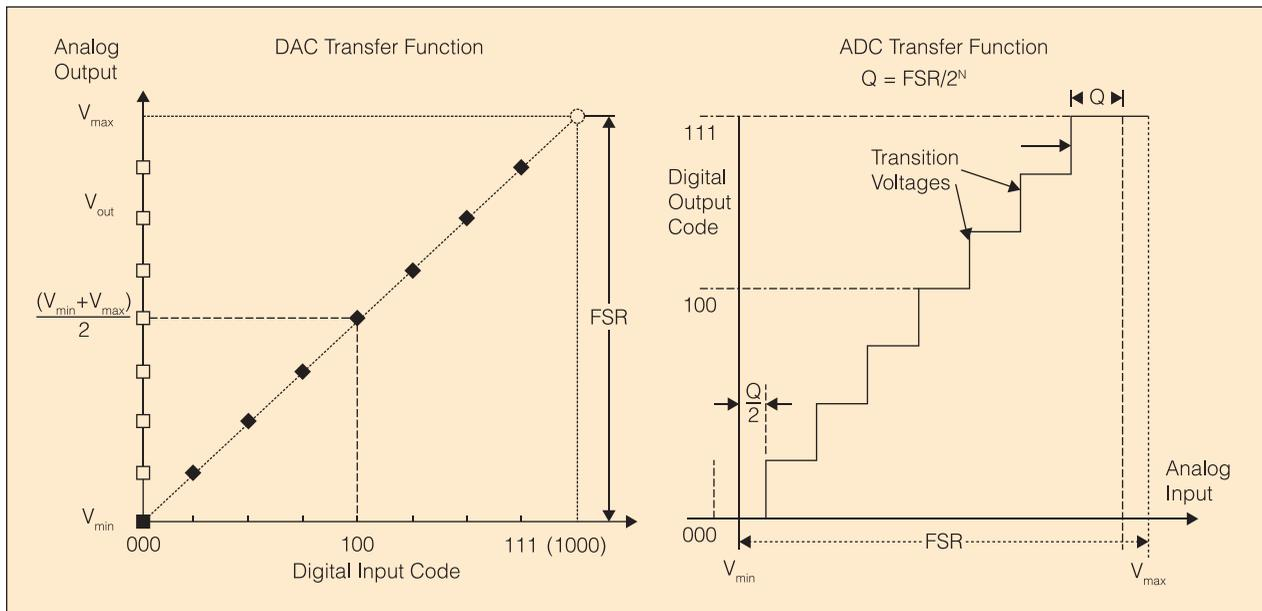
Fig. 3. Transfer functions of ideal 3-bit unipolar DAC and ADC (from [7], ©2020 IEEE).
