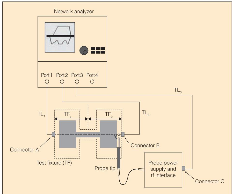
Fig. 4. Test setup for measuring the input impedance of single-ended stand-alone probe (from [7], ©2020 IEEE).
