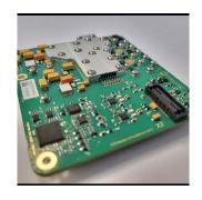
86 GHz) transceiver platform. Integrating all the RF transmit and receive functions required for an E-band radio link, the transceiver module offers a linear transmit power output of +23 dBm—3 dB higher than the standard Morpheus II product—while occupying the same compact footprint of  $90 \times 80$  mm. Receiver noise figure is typically 7 to 8 dB, and an enhanced option with 4.5 to 5.5 dB noise figure is also available for specialized applications.
