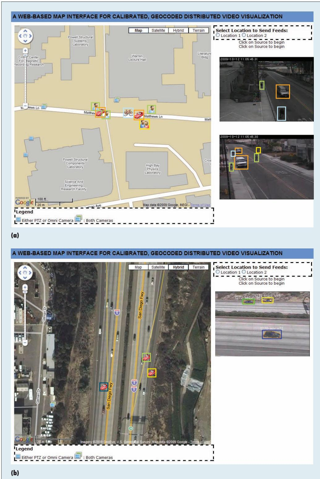
Figure 7. CANVAS visualization page. (a) A campus street is monitored using two slightly overlapping cameras. The output of object classification and tracking is marked on the map. Icons indicate the object type and are placed on the map based on camera georegistration information that converts image coordinates to GPS latitude and longitude. (b) Environmental context is presented using an aerial highway image. The detected vehicles are marked with car icons, which appear in the different lanes.
