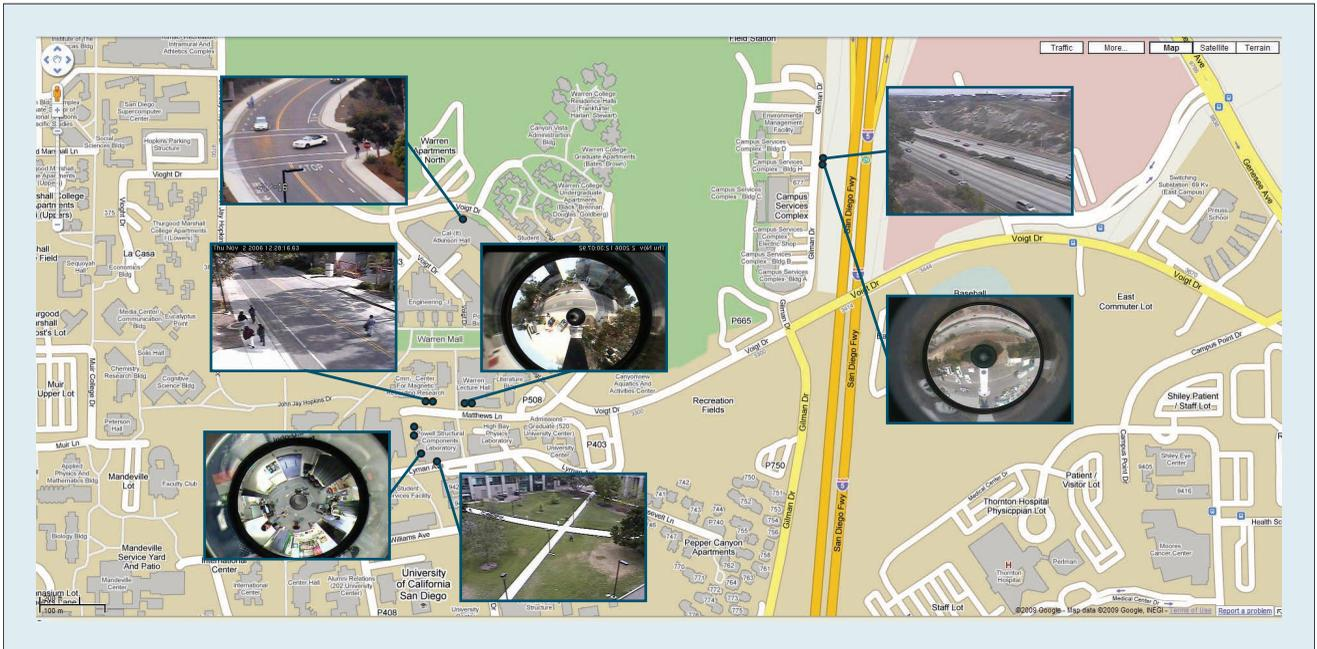
**Figure 2. University of California, San Diego video network.** A network of video cameras around campus provides coverage of different environments. Both rectilinear pan-tilt-zoom (PTZ) and omnidirectional cameras monitor highway vehicle traffic and the close interactions of people and vehicles on campus.
