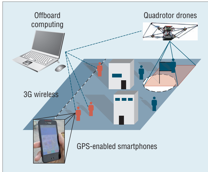
Figure 1. Stanford University researchers are developing technology that could let drones help capture-the-flag game players. The flying robots could identify important places in the playing area that humans can't see from the ground and the overhead locations from which the aircraft could observe them. An offboard computer collects players' GPS-based location data from their smartphones and then runs the algorithms.
