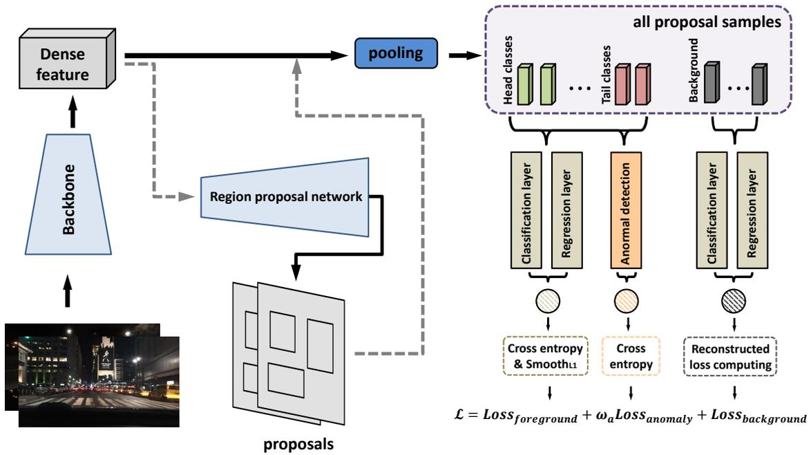
FIGURE 2: Overview of the proposed pipeline based on Faster R-CNN for night-time vehicle detection.
