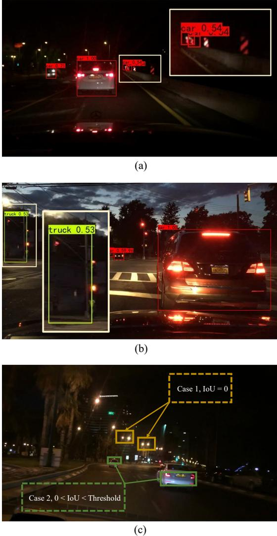
**FIGURE 3:** Illustration for the false detection cases. (a-b). Examples of false detection due to disturbance from interfering light sources. (c). Cases for the detected background proposals that may be misclassified during training.
