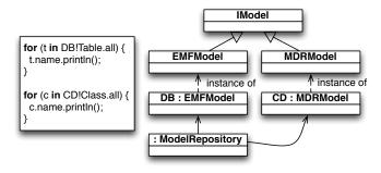
Fig. 3. Example of EMC Runtime Binding
