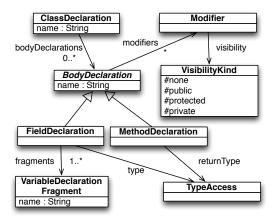
Fig. 4. Simplified view of the MoDisco Java metamodel
