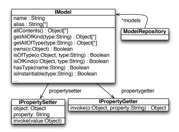
Fig. 2. The IModel Interface of the Epsilon Model Connectivity layer of Figure 1
