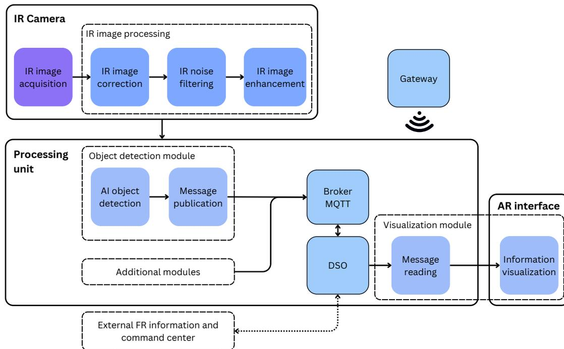
**FIGURE 1.** General architecture of the Smart Helmet. It is mainly divided into three devices interconnected between them, which are the IR camera, the processing unit, and the AR interface. Each of these components present inside the main operational modules that participate in the Smart helmet functions.
