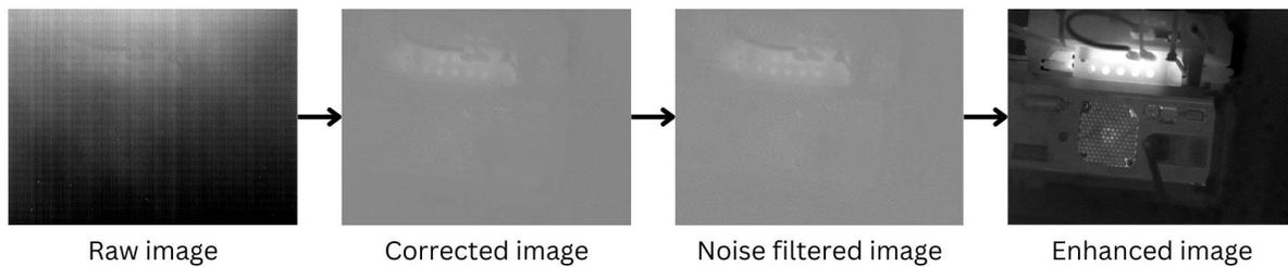
**FIGURE 3.** Example of the IR camera processing steps from the raw image captured by the sensor to the final enhanced image delivered by the camera.
