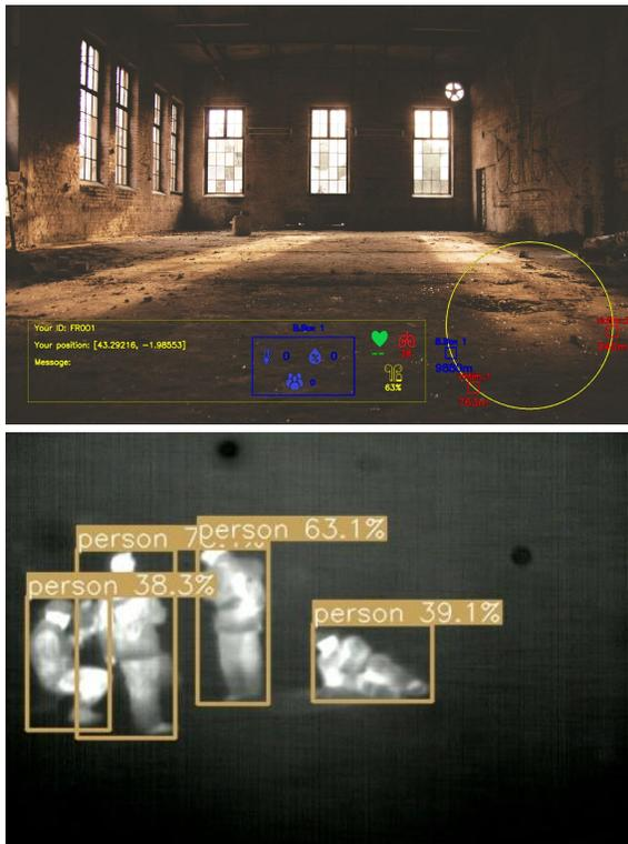
**FIGURE 4.** Examples of the smart visualization displayed on HUD. The upper part represents the visualization of the combined information on top of reality. The lower part shows the visualization of the thermal video stream with an object detection algorithm running on top, where 4 people are detected.
