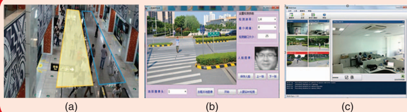
FIG 10 Intelligent video surveillance system. (a) Sparse degree test in subway, (b) real-time detection of pedestrian, and (c) tracking from multiple angles.
