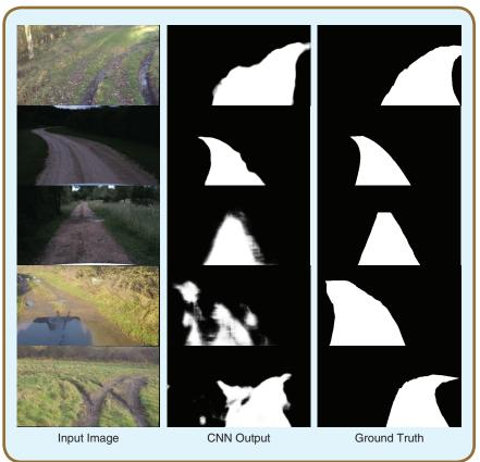
**FIG 3** Samples from our test data set. Rows 1–3: good results obtained respectively from FCN, Segnet and u-net; row 4: a poor result, possibly caused by shadows and water on the ground; row 5: an example of a fork in front the vehicle creating two valid paths, although our ground truth only includes the path that the vehicle originally took.
