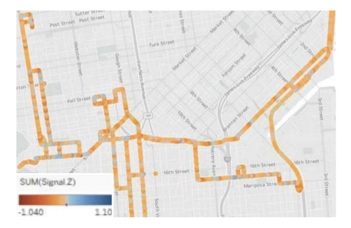
Figure 7: Longitudinal acceleration of a driver from cluster 2.
