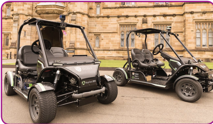
Electrical vehicles retrofitted with automation technology and logging capabilities.
