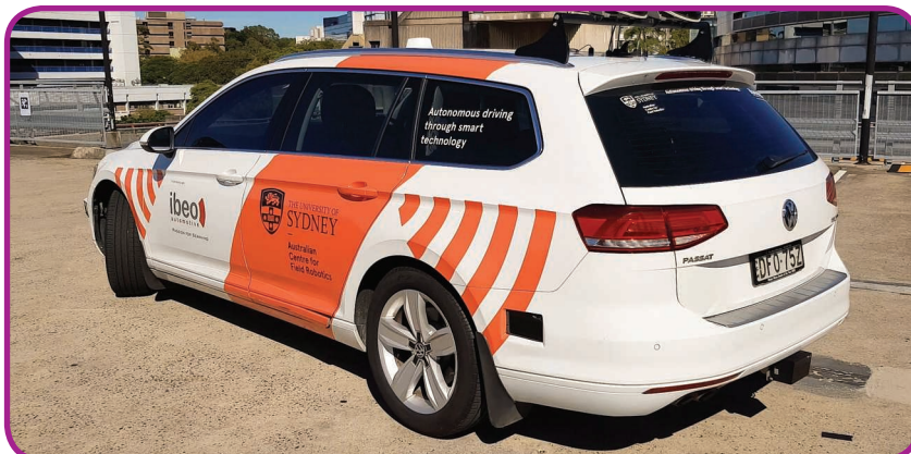
Urban vehicle retrofitted with 360 degrees perception, high accuracy localization and logging capabilities.
