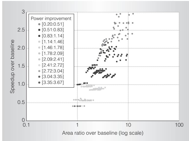
Figure 6. Multicore design-space exploration. The graph shows the average speedup for the six scientific kernels as a function of the area ratio over the baseline configuration, with the points gray-scaled according to the power improvement over the baseline.
