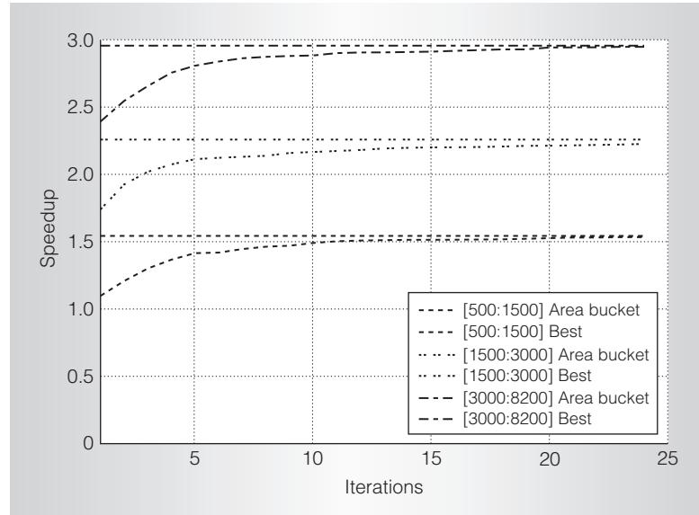
Figure 7. Convergence in the multicore design space. The multicore exploration quickly converges in 10 to 15 iterations.
