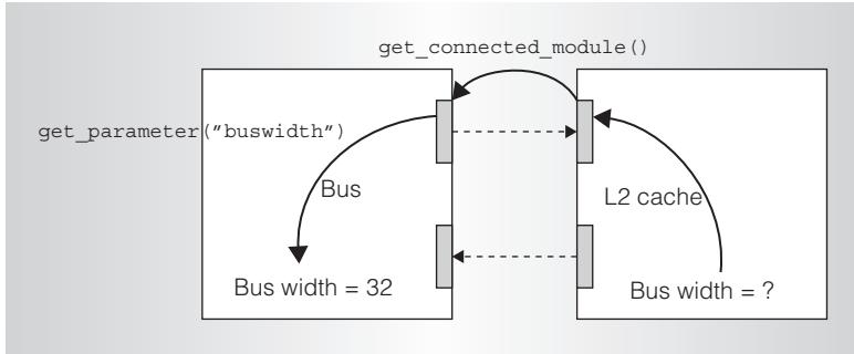
Figure 3. Self-configuration by probing connected modules. Modules have a parameter introspection interface API that lets other modules query its parameters through an interface.
