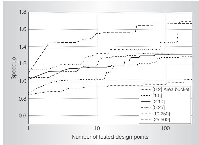
Figure 4. Convergence speed of statistical exploration. ArchExplorer achieves fast convergence through a genetic-like exploration algorithm.
