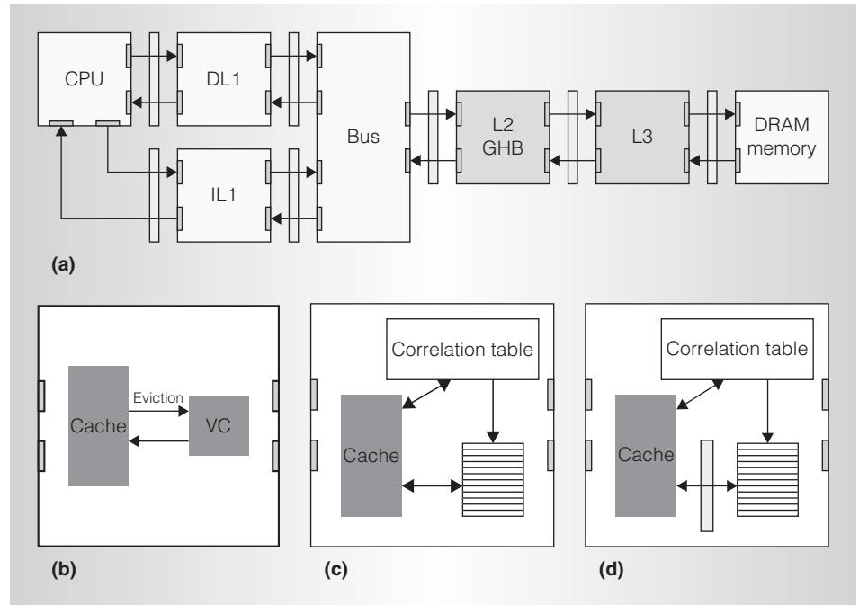
Figure 2. Modular simulation environment of ArchExplorer. Composing architectures (a) and fine-grained compositions: victim cache (VC) (b), time keeping (TK) (c), and prefetch buffer application communications interface (ACI) (d). (GHB: global history buffer)
