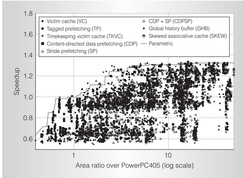
Figure 5. Parametric versus structural exploration. Advanced data cache mechanisms only moderately outperform an optimized standard data cache architecture.
