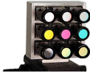
Fig. 1. A multispectral camera with nine channels [4].
