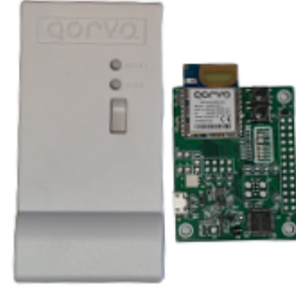
Fig. 1. Photo of a node of the proposed system, consisting of a DWM1001-DEV development board (right) with its casing (left).
