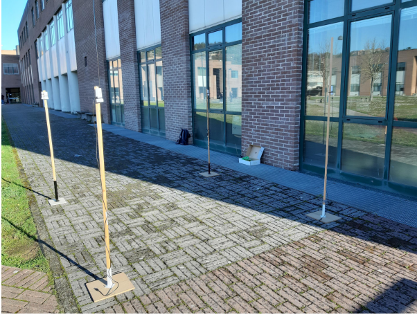
Fig. 10. Photo of the experimental setup. The four UWB nodes are mounted on stands and powered by battery packs.
