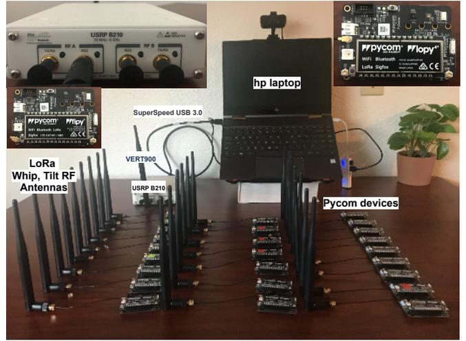
Fig. 1. Experimental LoRa device testbed.
