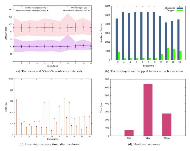
Fig. 6: Streaming recovery time during handover operation.
