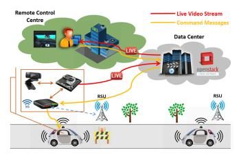
Fig. 1: Remote driving use case.
