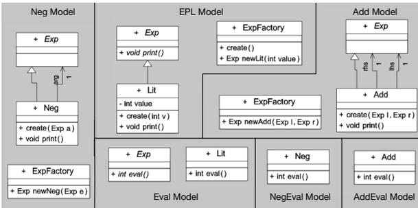
Fig. 3: Base UML Models for the EPL
