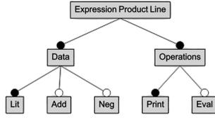
Fig. 2: The Feature Model for the EPL
