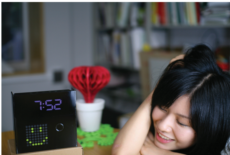
Figure 3. An alarm clock that won't shut off until the user smiles.
