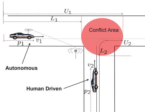
Fig. 1. **Two-vehicle Conflict Scenario.** Vehicle 1, whose longitudinal displacement and speed are denoted  $p_1$  and  $v_1$ , respectively, is autonomous and communicates with the infrastructure via wireless. Vehicle 2, whose longitudinal displacement and speed are denoted  $p_2$  and  $v_2$ , respectively, is human-driven and does not communicate with the infrastructure. A collision occurs when more than one vehicle occupies the conflict area at the same time.
