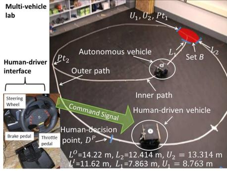
Fig. 3. Human-driver interface and roundabout system.  $L^o$  is the length of the outer path and  $L^i$  is the length of the inner path.
