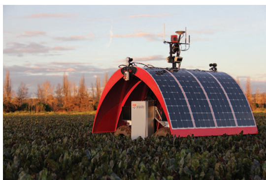
Figure 4. The Ladybird robot, designed for operation in vegetable crops, shown here at a field trial in Cowra, New South Wales. (Photo courtesy of ACFR, The University of Sydney.)
