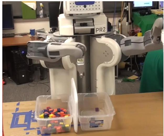
Fig. 17: PR2 executing the Box and Blocks Test.
