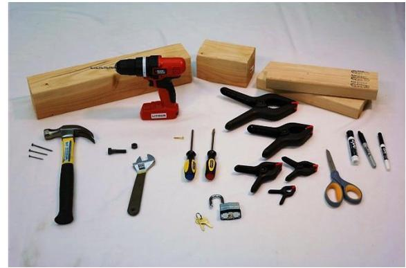
Fig. 3: Tool items in the YCB Object Set: back: wood blocks (four items, three sizes), power drill; front: nails (three sizes), hammer, plastic bolt and nut; adjustable wrench, wood screw, phillips and flat screwdrivers, padlock and keys, spring clamps (five sizes), scissors, markers (three sizes/types).
